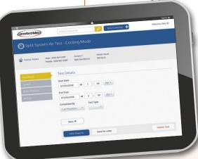
You simply collect four system pressures at the indicated locations. Lookup airflow on the appropriate fan chart for the equipment brand – or use our generic chart.
