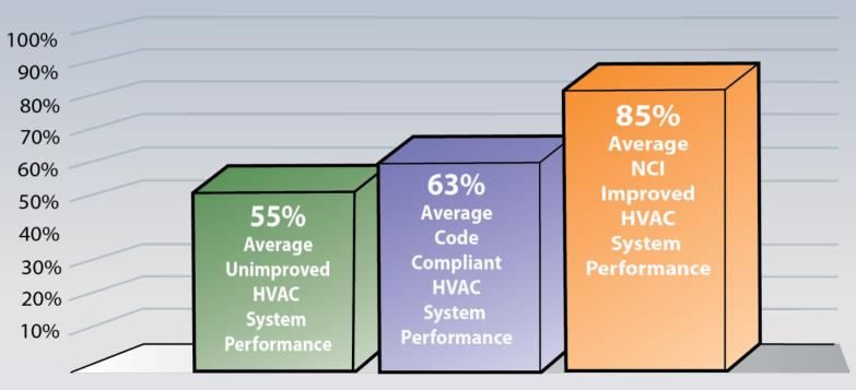
Average Percent of Rated System Capacity Delivered to Occupied Space Typical Existing, New Code-Compliant, and After Performance-Based Renovation
